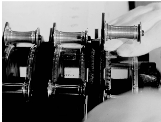
Illustration of how the synchronizer functions: each spool holds either the image strip or the film stock with the sound information, making it possible to synchronize them. See database entry.
