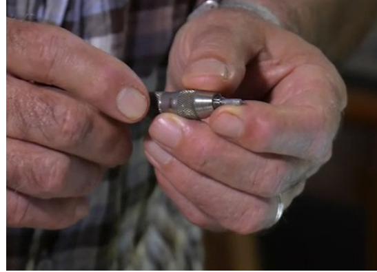
A carbide-tipped scriber used by Pierre Hébert to scratch his drawings onto black film stock. See database entry.
